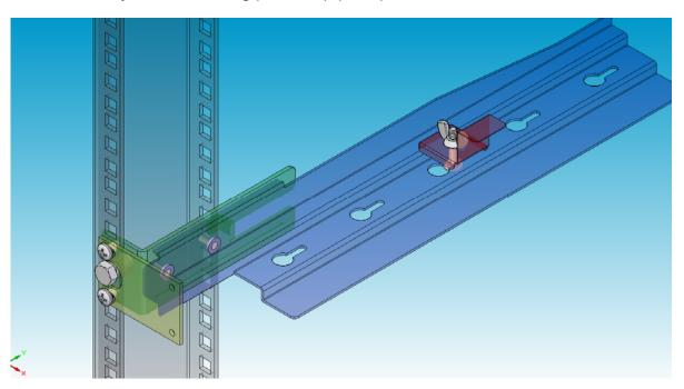
The bracket with flush mounted, equipment on.
