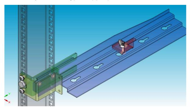
The bracket with offset installed equipment on.
